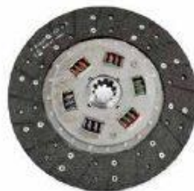
A conventional modern clutch plate, made in Germany. The kit can replace either 10in or 11in clutch plates; all other things being equal, the 11in plate and cover will last 10 per cent longer by virtue of a larger contact area
