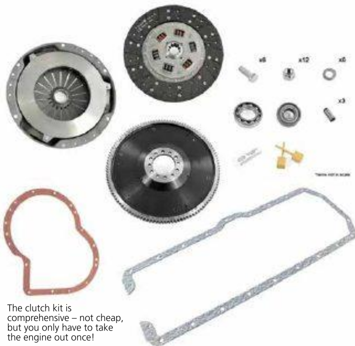
A new flywheel is the key to the clutch kit while a silky smooth finish and fresh ring gear are also not to be sneezed at. Different timing marks reflect right- or left-hand drive and have different access holes for the marks
