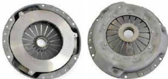
A conventional modern diaphragm clutch pressure plate
