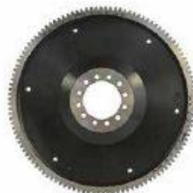
A new flywheel is the key to the clutch kit while a silky smooth finish and fresh ring gear are also not to be sneezed at. Different timing marks reflect right- or left-hand drive and have different access holes for the marks
