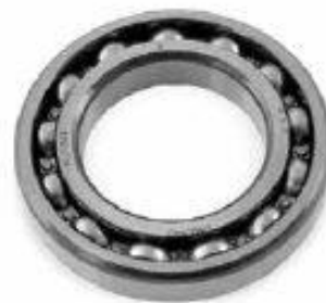
The new clutch release bearing, made in England and not Xinchang. Bonus!
