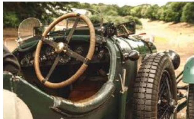
The hemp-wrapped, 20in steering wheel and scuffed cockpit sides showcase the patina that underscores the 4½'s originality
