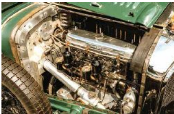
The 4.4-litre ‘four’ produced 130bhp, and a top speed of 90mph, in racing spec
