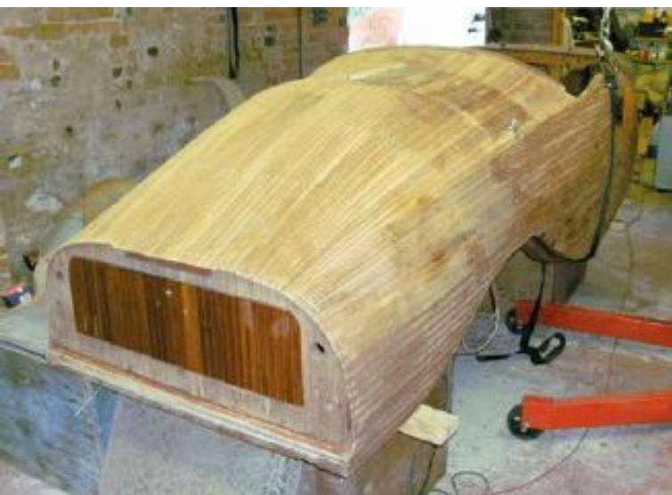
Renovation ongoing for the rear bodywork (above) and boot area (above right)
