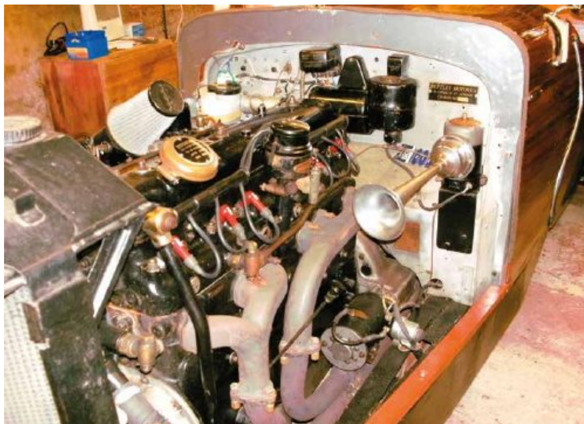
The original engine was replaced with an R Type 4½-litre unit married to a four-speed manual gearbox
