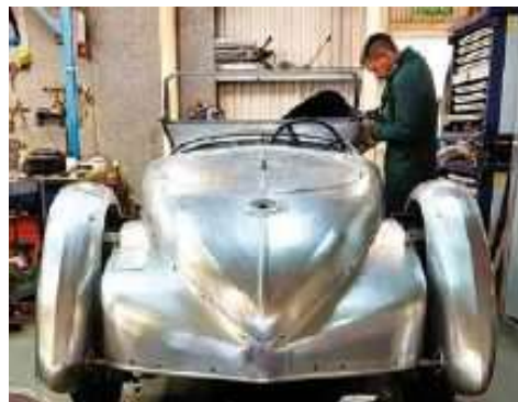
Bespoke Bodywork was tasked with carefully crafting the streamlined Ridlington-type shell for EYV 405
