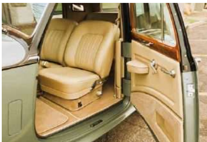
The new interior featuring a bespoke door panel, garnish mouldings, tilt-back seats and 'gooseneck' hinges
