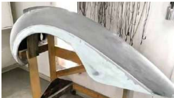
Swage lines were developed for the front wings to complement the rear-wing design
