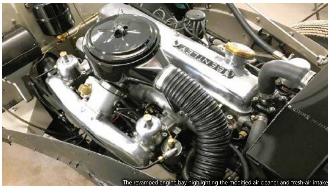
The revamped engine bay highlighting the modified air cleaner and fresh-air intake
