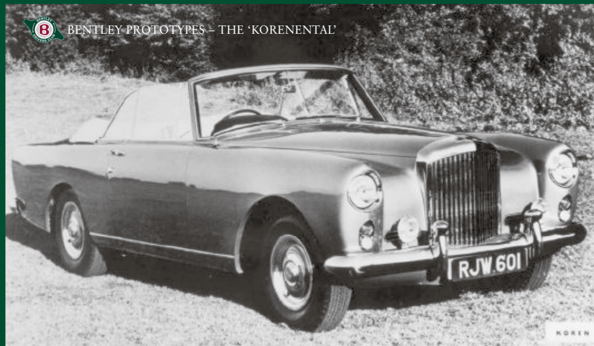
The production version of the S2 Continental DHC, with the finalised design for the front lamp housings
