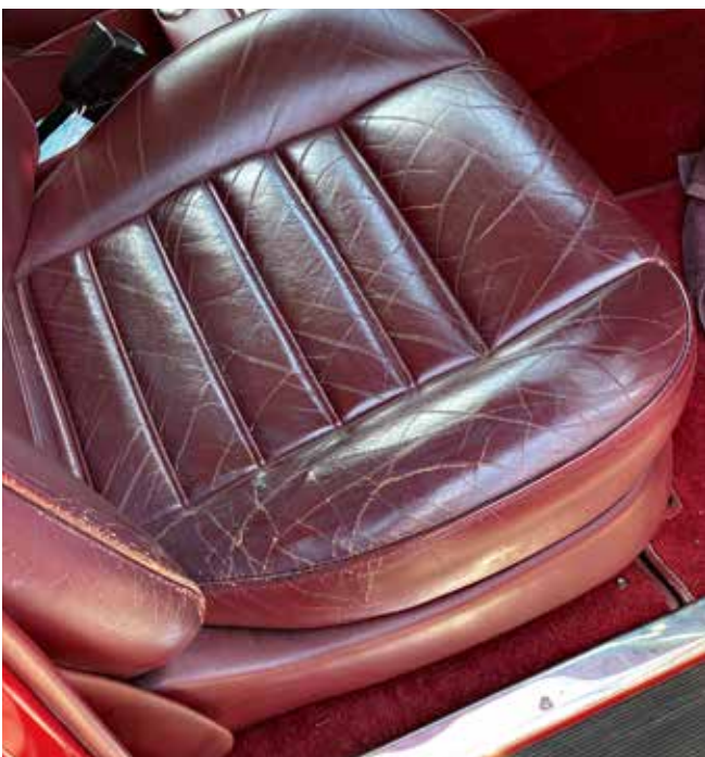
(above) Large cracks were apparent in the driver's seat before the restoration
