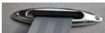
The rear parcel shelf, with aperture brackets, was bespoke manufactured
